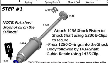
Attach 1436 Shock Piston to Shock Shaft using 5230 E-Clips
