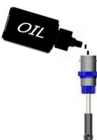
4) Place Bladder onto top of shock, small amount of oil should displace.
