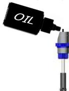
8) If the shock rebounds too fast, or you cannot push the shaft in until the ball cup gets close to the body, there is too much oil. Simply remove the Eyelet Cap and retighten the cap, typically this will allow just enough oil to escape to be successful without under-filling the shock.
