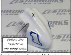
**Hood, Headers & Tank:** Follow the molded lines on the mold to cut the body parts out. Make body post hole (.200") on the "X". Drill a .125" hole on the dimpled dot on the headers marked with an "O".
