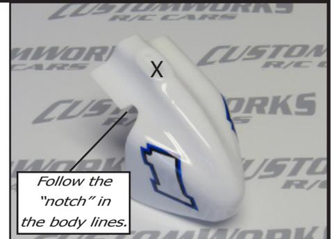
**Hood, Headers & Tank:** Follow the molded lines on the mold to cut the body parts out. Make body post hole (.200") on the "X". Drill a .125" hole on the dimpled dot on the headers marked with an "O".
