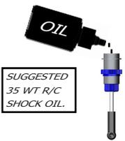
2) Slowly move the shaft up and down several times to allow air bubbles to escape to the top.
