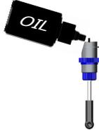
8) If the shock rebounds too fast, or you cannot push the shaft in until the ball cup gets close to the body, there is too much oil. Simply remove the Eyelet Cap and retighten the cap, typically this will allow just enough oil to escape to be successful without under-filling the shock.
