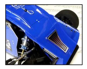
3. Side panels — install side panels on the cage (you will have to remove some of the screws already installed). Trim the side panels to clear the rear shock tower as shown. The left side panel will also need trimmed to clear the motor.
