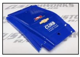
2. Nose piece – Cut as shown and drill 1/4" hole on the rear dimple as shown (do not follow trim lines).
