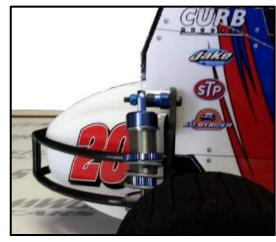
4. Headers – trim headers and drill (2) .125 mounting holes on each. Mount as shown.
