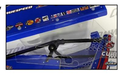
7. Front wing — Assemble the front wing and mount to the front nerf bar as shown.
