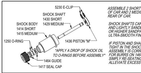
ASSEMBLE 2 SHORT SHOCKS FOR FRONT OF CAR AND 2 MEDIUM SHOCKS FOR REAR OF CAR
