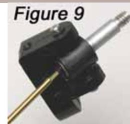
**Step #4:** Press the Pivot Ball into the #5228 Ball End, then thread the Ball Ends onto each end of the #5221 Turnbuckle. When completed it should look like the Camber Links in **Figure #11**.
