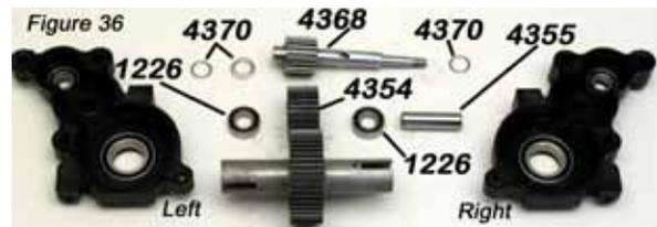
Half. Press (2) #1226, 3/16" X 3/8" Bearings into each side of the #4354 Idler Gear and slide that onto the Idler Gear Shaft. Now install the Right Side Diff Hub (Hub with Diff Bolt) into Right Transmission Half. Finally place (1) THICK and (1) THIN Washer on the short shaft on the Top Drive Shaft and align the entire Left Side Transmission Half over all 3 gears.
