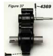
**Step #3:** Install (1) 3/8" FH Screw into the very bottom of the Left Side Transmission Half as shown in **Figure #37** and thread it in until it is tight. Press the #4369 Roll Pin into the hole in the Top Gear Shaft so that equal parts of the Roll Pin stick out of the axle, just as when installing the Roll Pins on the CVD axles.
