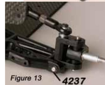
**Step #7:** Pass one 4-40 X 1/2" FH Screw thru the front of the Shock Tower in the upper camber link hole. On the backside of the Shock Tower, slide (1) #5212 Washer and then the Ball End from the Camber Link onto the 3/8" FH screw. Fasten to car by threading on (1) #5205 4-40 Locknut. The finished assembly should look like that in **Figure #14**. Repeat for other side of car.
