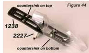
**Step #5:** Hold the #1238 Transmission Brace as shown in **Figure #44** by taking note of the position of the entire part by looking at "square" in the center of the piece and which side the countersunk holes are positioned. Holding the part as shown in **Figure #44**, Install (2) 1" SH Screws into the middle set of holes on the Transmission Brace. Slide the #2227 Transmission Brace Spacer over the 1" Screws.
