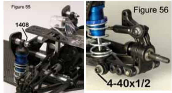
**Step #10:** Mount the Front Shocks by placing the Shock Cap End of the shock onto the mount on the Shock Tower. Insert (1) #1408 Shock Bushing on the mount and into the Shock Cap and fasten with (1) 4-40 Lock-nut as shown in **Figure #57**. Mount the Eyelet end of the Shock in between the supports in the Suspension Arm with (1) 5/8" SH Screw.
