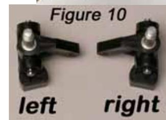
**NOTE:** The Turnbuckles have *normal* threads on one side of the turnbuckle, and *reverse* threads on the other. Mark the Ball End with the NORMAL threads so you remember which way to turn the Turnbuckle for adjusting the Camber Link with supplied tie-rod wrench.
