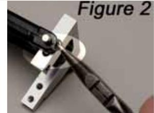
**Step #2:** Repeat Step #1 with #3250 Suspension Arm facing opposite direction from Suspension Mount. This will make a Left and Right side front suspension for the car.
