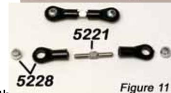
**Step #5:** Attach the Camber Link by sliding a 1/2" BH Screw thru the Ball End, followed by (3) #5212 Washers, then screw into the top of the Castor Block as shown in **Figure #12**.
