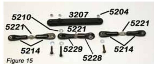
**Step #3:** On the remaining turnbuckle thread one #5228 ball end and one #5229 ball end, these are the two shortest ends in the bag. Now install the Servo Linkage to the raised hole on the #3207 Steering Rack Slide using (1) 1/2" 2-56 SH Screw with (1) #2 Washer on each side of the Ball End. Insert (1) 2-56 Locknut into the hexagon hole on the backside of the #3207 Steering Rack Slide and tighten the 1/2" 2-56 SH Screw to it. Refer to **Figure #15** for example.
