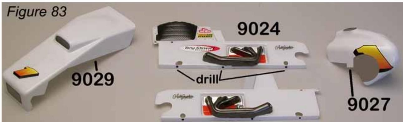
**Step #7:** Using **Figure 83** as a guide trim, and paint the #9024 Body Panels, #9029 Eagle Hood, #9027 Tail Tank on the molded body lines for either REAR or MID-MOTOR set-up as directed...
