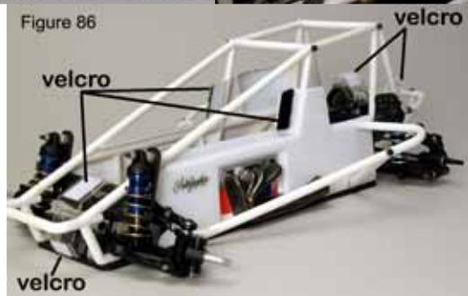
**Step #9:** Following **Figure #86**, mount one side of the Velcro to the places shown. We suggest to mount the "hook" side of the Velcro to the body mounts on the car.
