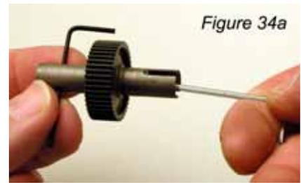
Pay attention to feeling when the spring is fully compressed, you DO NOT WANT TO OVERTIGHTEN THE BOLT. When the spring is fully compressed, loosen the Diff Bolt 1/8 of a turn, No more or less. Your Diff should spin smoothly with the hubs turning in opposite directions.
