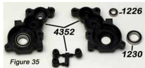
**Step #1:** Separate the #4352 Transmission Halves from the each other, and insert (1) #1226, 3/16" X 3/8" Bearing to the top of each case and (1) #1230, 3/8" X 5/8" Bearing to the bottom of each case as shown in **Figure #35**.
