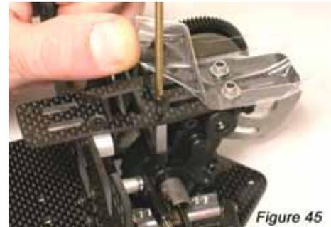
**Step #8:** As shown in **Figure #45**, gently pull the Tail Tank Mount to one side and use a 3/32" Hex Wrench to tighten the 1" SH Screw to the Transmission Casing.
