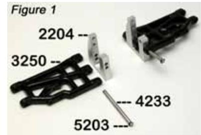
**Step #2:** Repeat Step #1 with #3250 Suspension Arm facing opposite direction from Suspension Mount. This will make a Left and Right side front suspension for the car.
