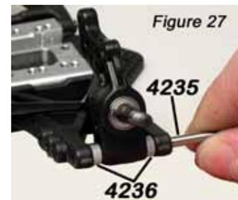
**NOTE:** There are extra .010" thick Shims enclosed, these are to be used if the Rear Carrier Shim does not take out all of the play. You want the Bearing Carrier to be free as it pivots on the pin, but not slide forward/backward on it excessively. Also the Bearing Carriers can fit on either side of the car; this is no RIGHT or LEFT side to this part.
