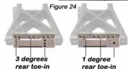
**NOTE:** More Toe-IN increases rear traction while hurting straight line speed. Less Toe-IN decreases rear traction while improving straight line speed.
