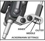
ACKERMANN IS THE DIFFERENCE THE FRONT TIRES ROTATE DURING STEERING INPUT. TYPICALLY YOU CAN USE THIS ADJUST-MENT BY MOVING THE LF LOCATION ONLY.
