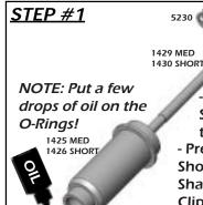
**BUILD 2 SHORT & 2 MED** LENGTH SHOCKS! USE #1429 SHAFT WITH #1425 BODY USF #1430 SHAFT WITH 1426 BODY .
