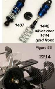
Step #8: On the Front Shock Tower, Insert (1) 4-40x7/8" SH Screw thru the upper hole on each side of the Shock Tower as shown in Figure #54. Thread on (1) #2214 Shock Stand-Off onto each screw with the shoulder on the spacer facing AWAY from the Shock Tower.
