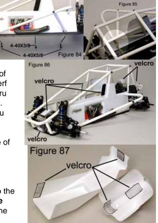
**Step #11:** Assemble the #9021 Wing kit using the instructions provided in the wing bag. Mount the wing to the car and it should now look just like the car shown below.
